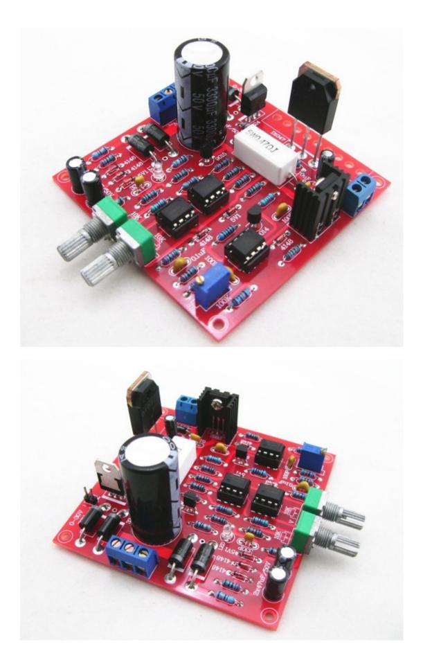
The potentiometer can be installed directly on the board, or with socket and wires. You may also replace it with multiturn potentiometer, which makes adjustment more precise.
