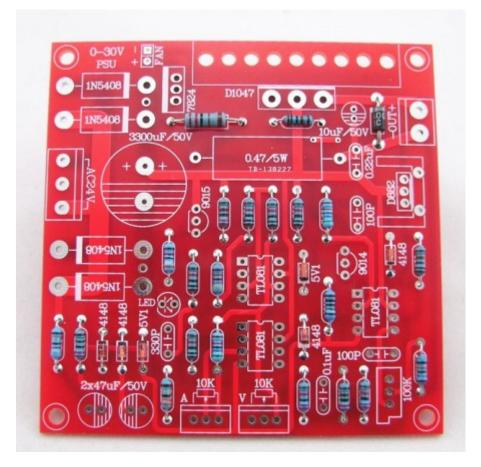
Install other component in accordance with the principle that from largest to smallest, lowest to highest.
